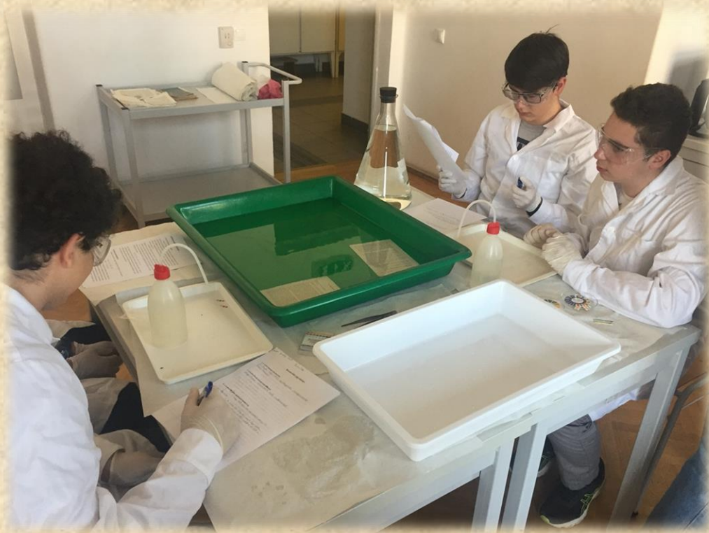
After washing them in warm water, we transferred the sheets into a \text{Ca}(\text{OH})_2 solution in order to deacidify them.
