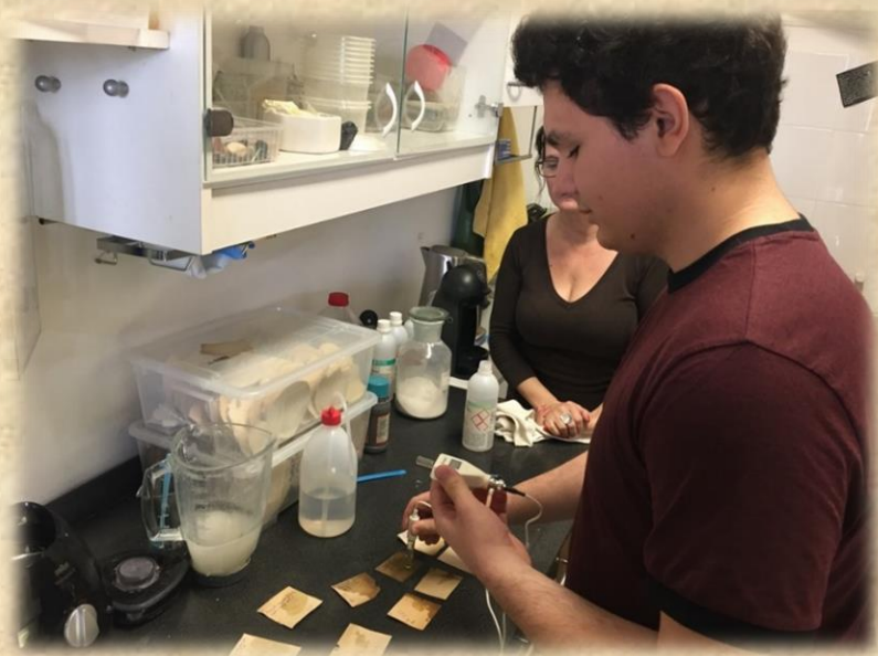
Zsolt is measuring the pH value of old pieces of paper using a portable pH meter.
